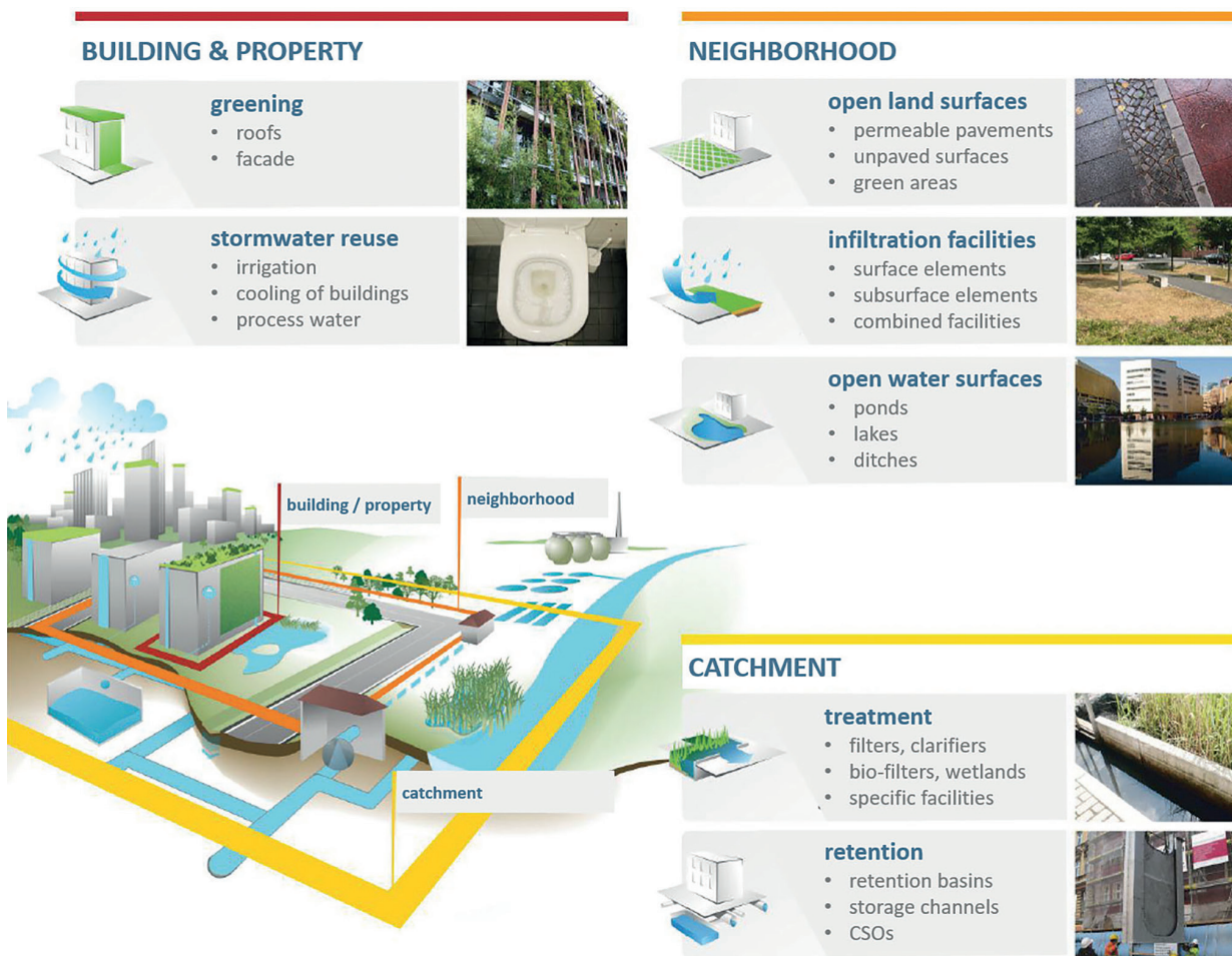
Figure 3 Overview of Sponge City Elements (based on Matzinger et al., 2017) 图 3 海绵城市元素概览 (基于 Matzinger 等, 2017)
